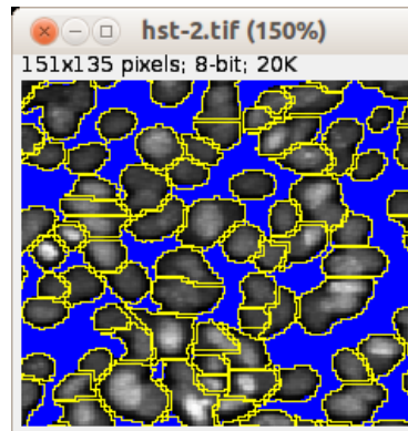
Figure 8.5: Segmentation of the nuclei with the watershed algorithm.
