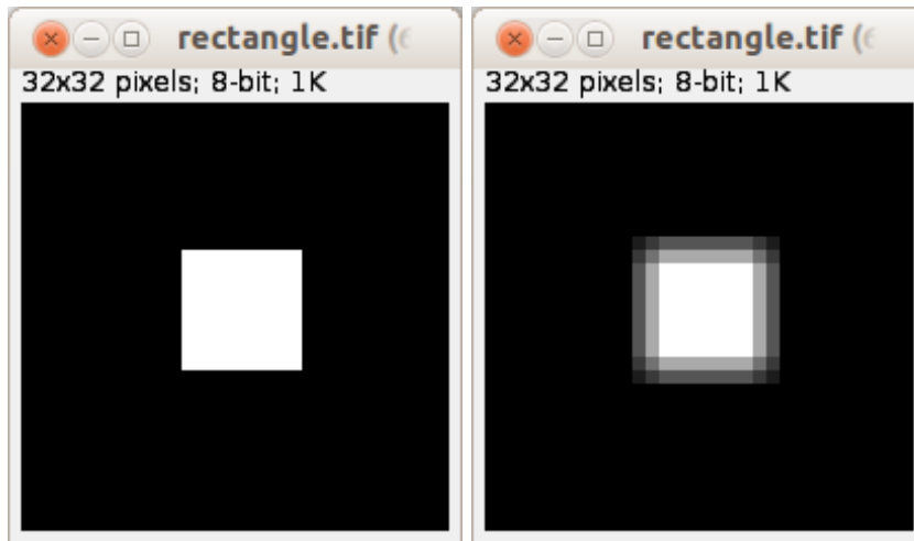
(a) A white rectangle. (b) The white rectangle after applying a mean filter of radius 1.
