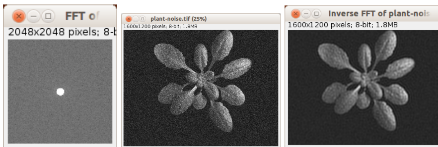
(a) Using clear instead of fill lets the corresponding frequencies pass. (b) The original plant noise image. (c) The image after filtering in the frequency domain.
