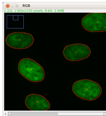
(a) Detail of the overlay of the original image and the outlines of the particles taken into account by the particle analyzer.
