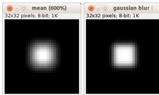
(a) Mean filter with radius 3 applied to the rectangle image. (b) Gaussian blur filter with \sigma = 1.2 applied to the rectangle image.
