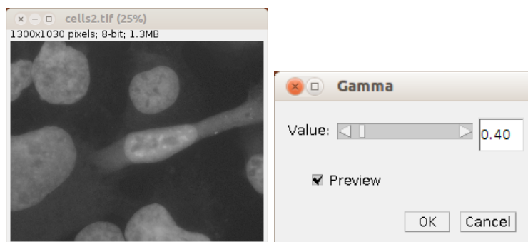
(a) A gamma adjustment has been applied to the image. (b) The gamma adjustment dialog.
